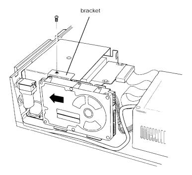
6. Secure the mounting plate with the screw, as shown above.
